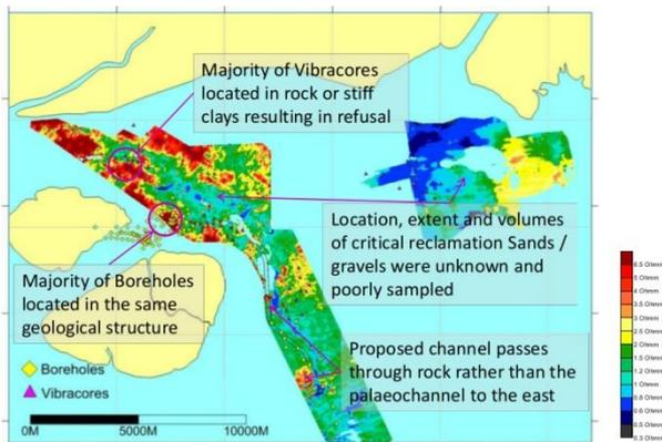
Figure 5. In this study, a geotechnical campaign was undertaken to map the geological structures. A subsequent Aquares study determined that the layout of geotechnical sampling sites did not cover the geological structures present. Failure to do this early in the project, resulted in millions of dollars of geotechnical studies that did not satisfy project aims, significant lost time and many millions of dollars in potential cost over-runs.
