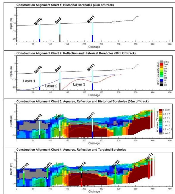
Figure 4. Here is an analysis of cross sections of boreholes and boreholes combined with two and three dimensional geophysics. In the top diagram three historical boreholes are seen that are up to 40m off track, no rock is evident. In the middle diagram, two dimensional quantitative geophysics is added, again, no rock is obvious. In the lower diagram, three dimensional Aquares geophysics is added and a high resistivity structure is seen that is subsequently drilled and found to be rock.
