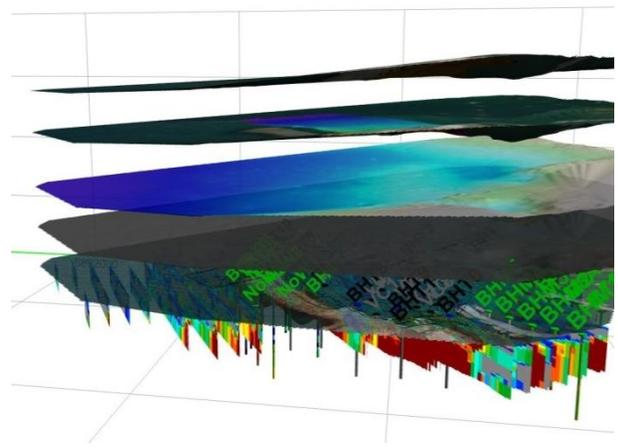
Figure 6. A 4 dimensional ground model in a GIS framework that includes: Aquares; Historical Boreholes; new targeted boreholes; vibracores; bathymetry; Magnetometer; reflection and sidescan sonar data. In this model, the continuous Aquares data provides the base structural data that is supported by a limited number of targeted boreholes and the findings of the historical datasets.
