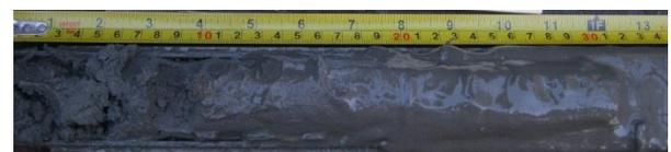
Figure 3. A typical split spoon (disturbed) sample recovered as a result of an Standard Penetration Test.
