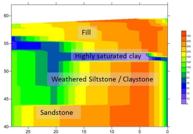
Figure 10. A thin, highly saturated clay layer is seen in the cross section of the slip region. Findings were later confirmed utilising boreholes and the clay layer was detected as the geologist was looking for the layer.
