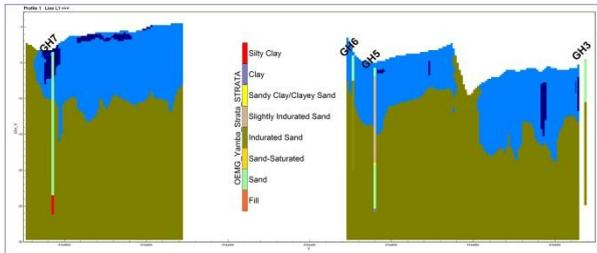
Figure 8. It can be seen from a cross section along the centre line that boreholes GH6 and 3 conform to the predictions of the Aquares model, but GH5 and 7 do not. However, after reviewing the original borelogs and in particular the SPT values, the client was able to re-interpret the findings of the boreholes to conform to those of the Aquares model.
