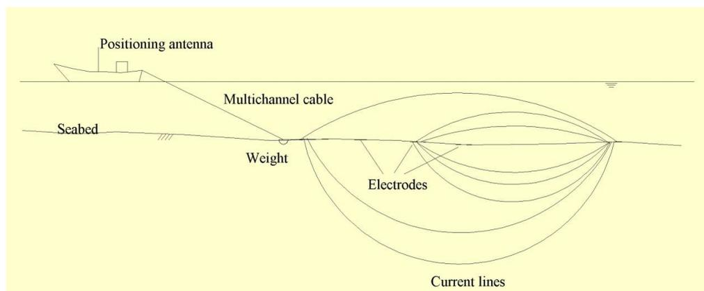
**Figure 2 Principles of Vertical Electrical Sounding – On water**
