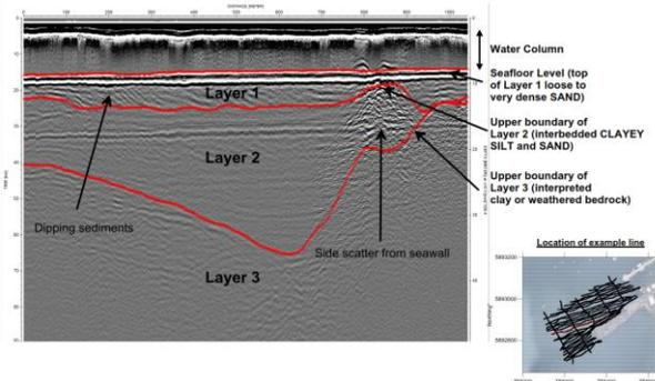
Figure 5 Interpreted reflection results from the 2014 GBG geophysical campaign [5].
