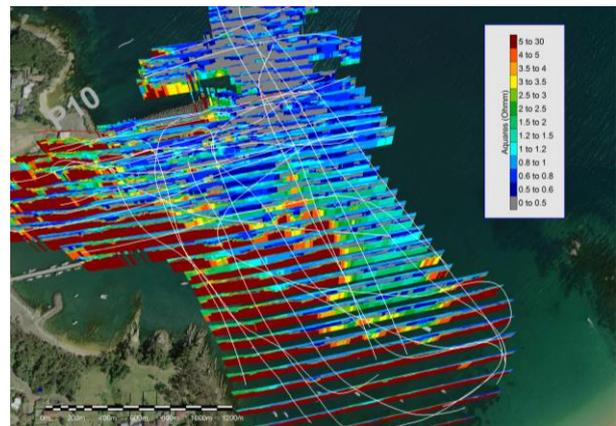
Figure 4 An initial review of the IDGM is made up of 16 line Kilometres and over 9000 shot points of data and sees complex high resistivity structures evident in the shallows to the north and east of the survey site deepening to the south.
