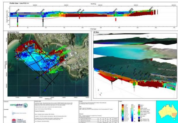
Figure 7 The IDGM is a digital chart delivered to the client with free viewer software. The chart contains a 4D view, a 2D plan view with grids that can be turned on and off as well as vertical sections along agreed flight lines that can be cycled through.
