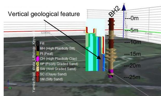
Figure 2 OEMG has been able to utilise Aquares results to identify isolated geological structures that may cause problems during construction. In this figure, an unusually soft vertical structure (dark grey) was found to persist to the limit of vertical detection of the Aquares cable utilised. The area was then tested with a borehole and characterised by very low SPT values and would have been problematic for the Horizontal Directional Drill proposed. Data courtesy Clarence Valley Council.
