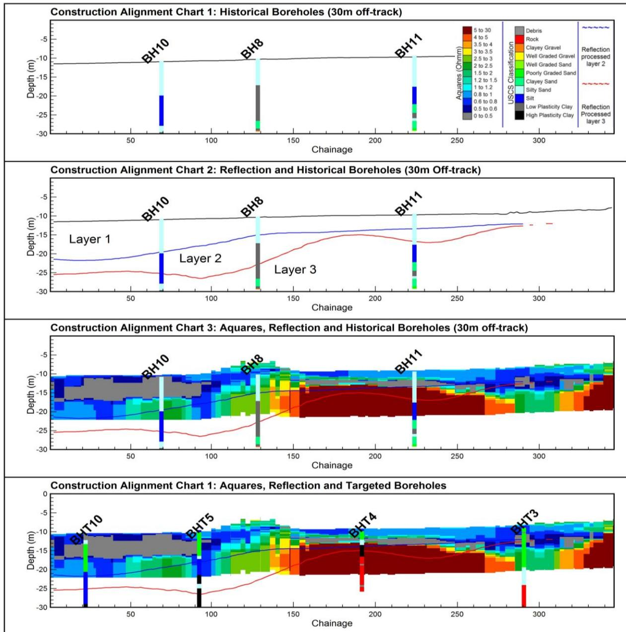
Figure 8 An analysis along section line “P10” looks at the application of different datasets and how they change the interpretation and influence construction.
