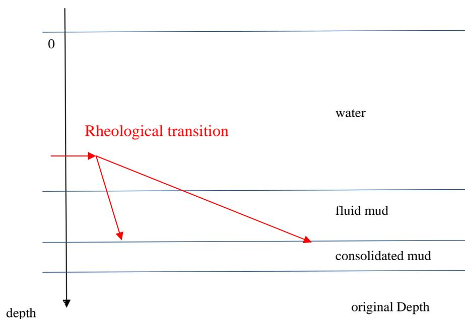
This distinction between fluid mud and consolidated mud, made possible by this sounding method, is very important and cannot be obtained by the actual sounding methods in use.
